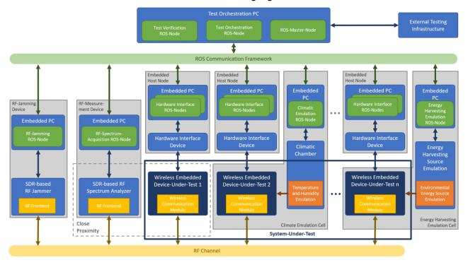
Figure 16 Wireless embedded device testbed architecture based on ROS
