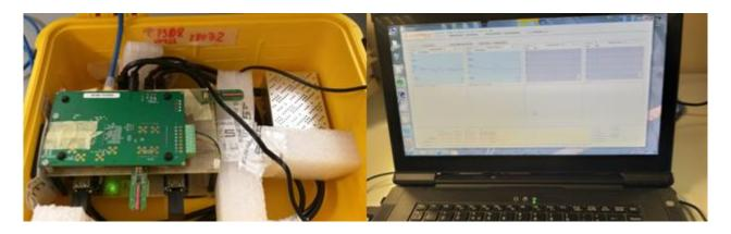
Figure 55 Magnetic sensor prototype (left) and control console (right)
