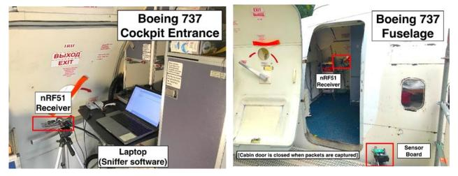
Figure 8 Sensor wireless signal transmission experimental setup inside a Boeing 737 fuselage
