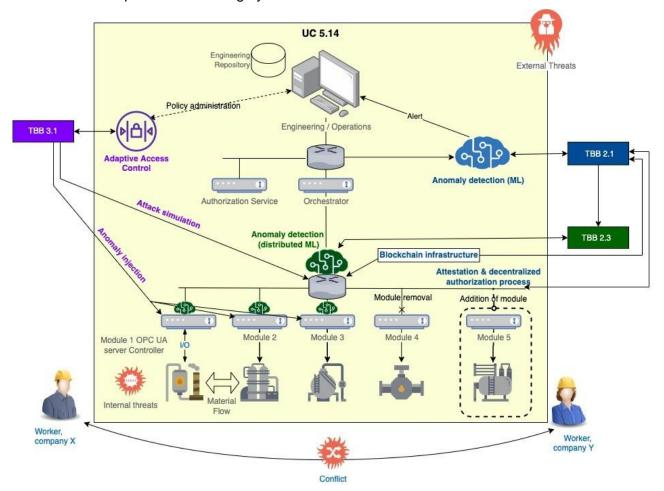
Figure 112 High-level architecture of the Use Case and connections with TBBs
