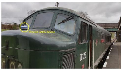
Figure 89 Installation of the GNSS equipment for enhanced reference positioning data
