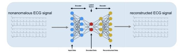
Figure 66 Anomaly detection principle
