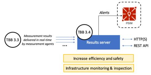
Figure 33 Simplified functional flow of data
