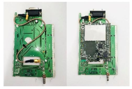
Figure 98 RFID Reader Prototype
