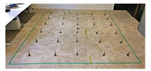
Figure 14 A network of 30 energy harvesting nodes and a gateway in a 4 m by 4 m area emulating multiple harvester events per second for showing TUD's MAC protocol
