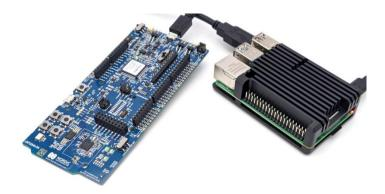
Figure 17 Embedded host node (Raspberry PI) and connected device-under-test (nRF52840 development kit)
