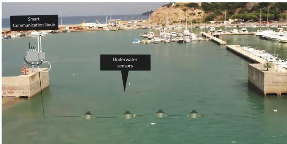
**Figure 52 Underwater sensors and a multi-interface node used to monitor passages through harbour entrance channel**
