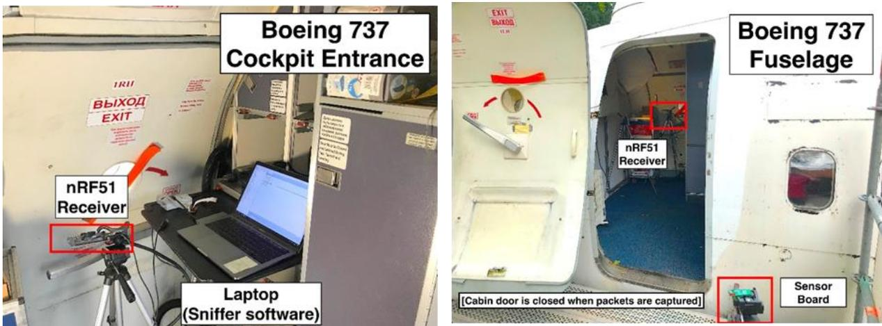
**Figure 8 Sensor wireless signal transmission experimental setup inside a Boeing 737 fuselage**
