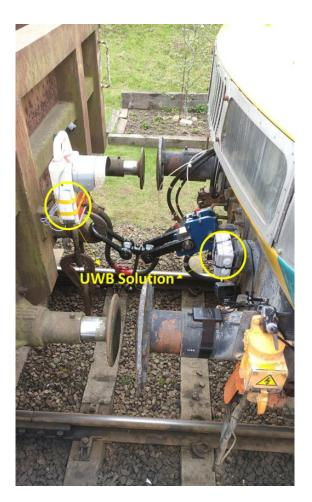
Figure 88 Installation of the UWB solution for proximity detection
