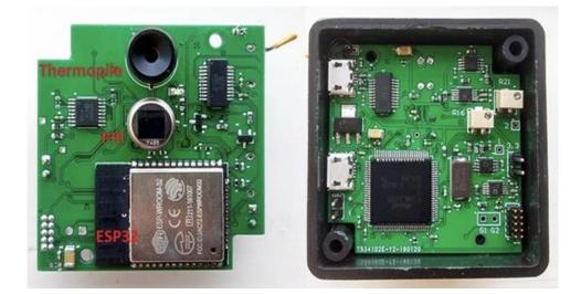
Figure 76 PIR/Thermopile localization module with case
