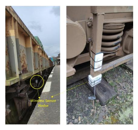
Figure 87 Installation of the Wireless Sensor Nodes in the rolling stock
