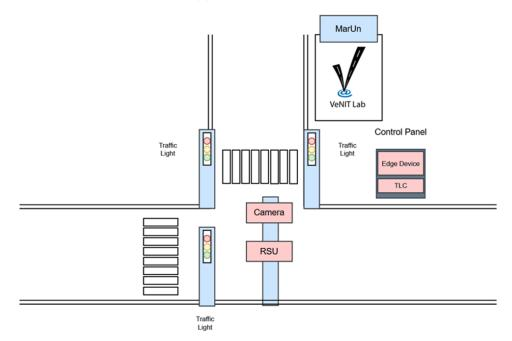
Figure 104 Layout for Marmara University Smart Intersection Testbed
