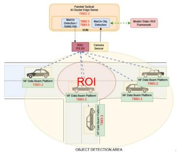
Figure 107 Smart Intersection infrastructure and BBs mapping
