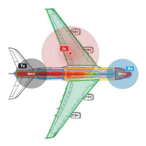
Figure 3 Real life situation in the WAIC system. Transmitting device (Tx) mounted in the back of the airplane may encounter problems while communicating with receiver (Rx) because of intentional interference created by a jamming device (Jx) mounted outside of the outside of the airplane
