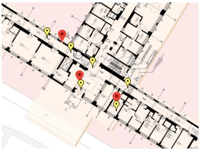
Figure 75 Installed Gateways (yellow markers) in Copernicus Medical Facility, which detects medical equipment (red markers)
