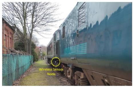
Figure 86 Part of the train composition, and one of the installed wireless sensor nodes
