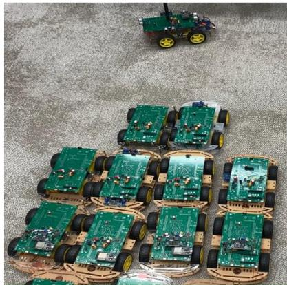
**Figure 1 Autonomous cars fabricated as part of the robotic testbed**
