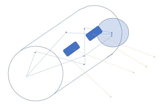
Figure 4 WAICs 3D channel model (multi-ray and stochastic geometric) for avionics communications
