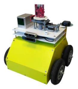
Figure 101 Mobile platform equipped with the sensor's payload
