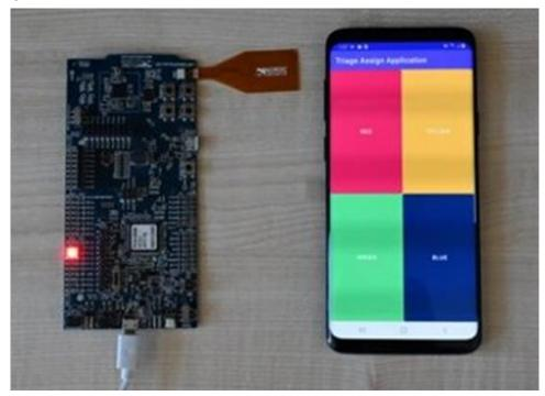
Figure 74 nRF board with Android triage App for MCI triage handling
