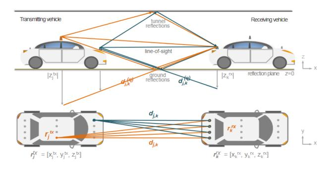
Figure 2 V2V platoon MIMO model inside a semi-circular tunnel (lateral view)
