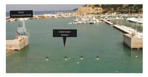
Figure 52 Underwater sensors and a multi-interface node used to monitor passages through harbour entrance channel
