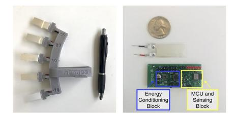
Figure 13 Wireless and battery less avionics sensor, called Hermes that simultaneously enables piezoelectric energy harvesting as well as sensing
