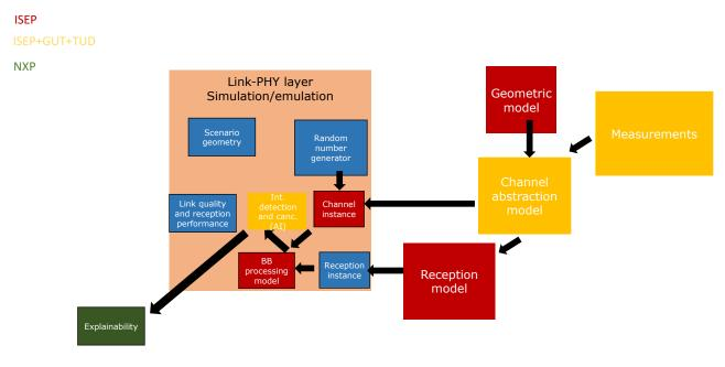
Figure 7 Simulator used by ISEP to use interference and channel measurements to evaluate the use of AI for interference detection and cancellation
