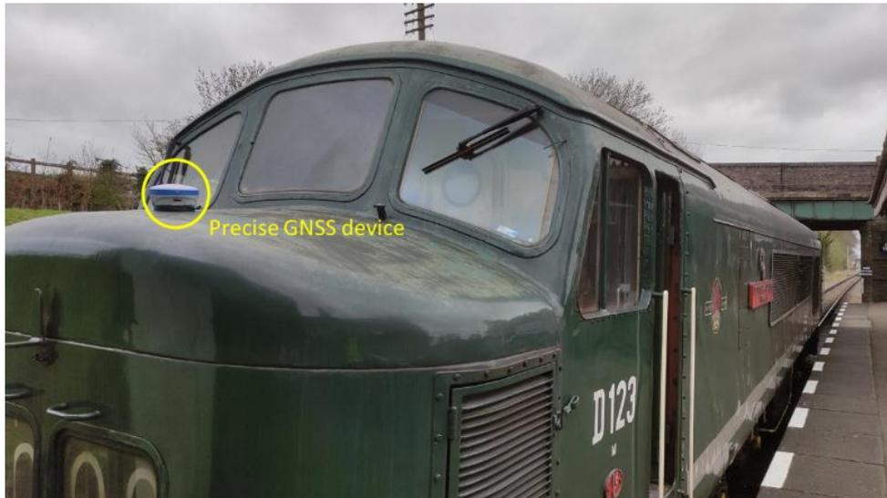
**Figure 89 Installation of the GNSS equipment for enhanced reference positioning data**
