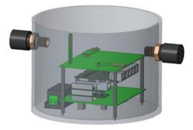
Figure 122 The design of the Magnetic sensor node
