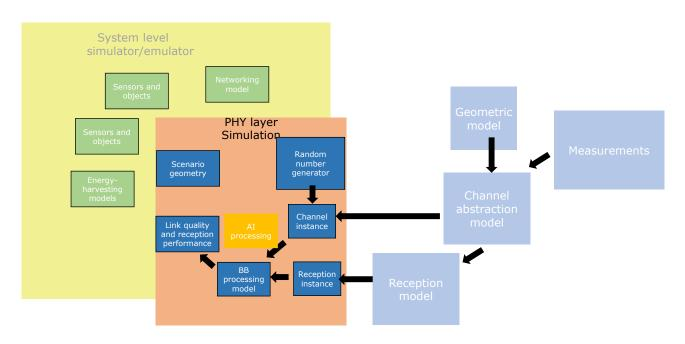
Figure 12 Simulator used by ISEP to provide simulations of battery-less devices with energy harvesting capabilities in WAICs networks
