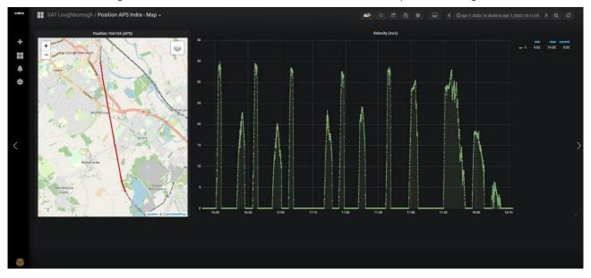
Figure 85 Dashboard showing INDRA's WSN GPS and accelerometer data reported during the tests
