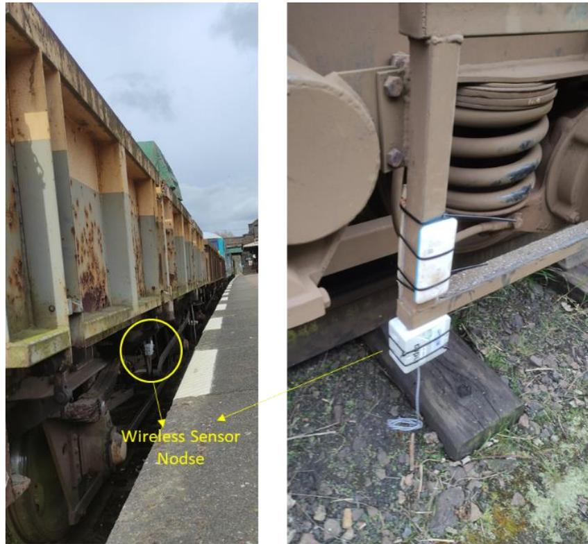
Figure 87 Installation of the Wireless Sensor Nodes in the rolling stock
