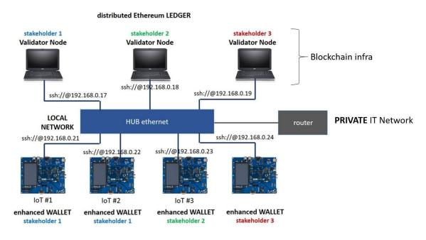
Figure 114 Decentralized network deployed for the Demonstrator B
