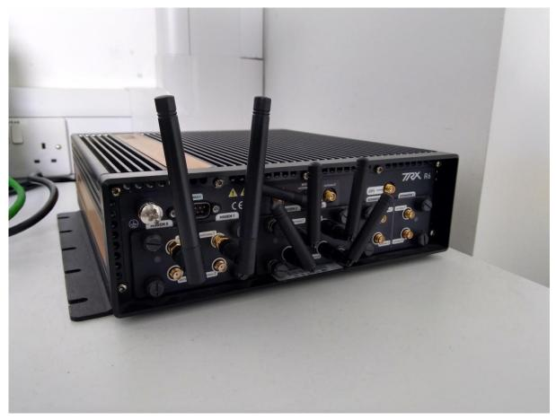
Figure 90 TRX R6 gateway computer with multiple modems
