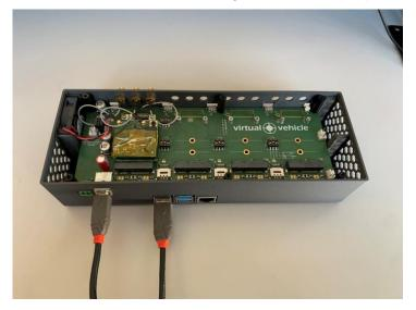
Figure 106 Vehicle CAPTAIN - Hardware with communication module carrier. Equipped with an ITSG5 module in the picture
