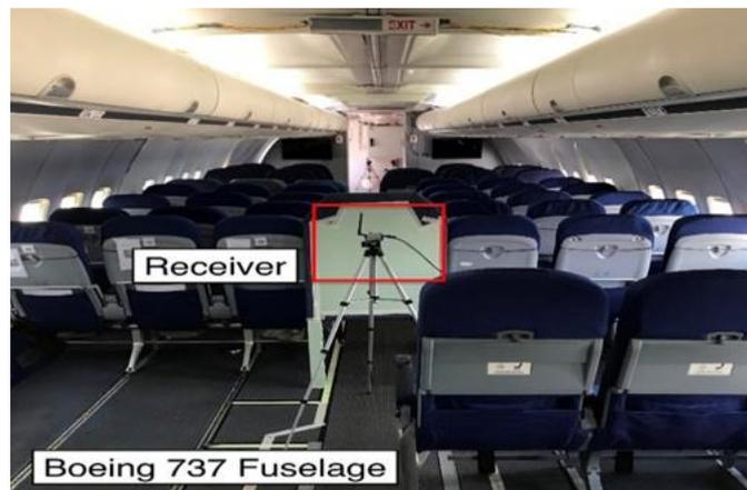
**Figure 15** Experiment setup inside fuselage to test energy harvesting MAC protocol
