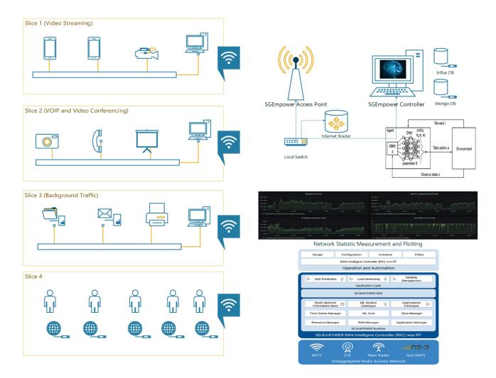
Figure 67 AI based wireless access point control structure
