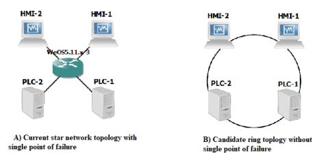
Figure 111 Network topology update of demonstrator A
