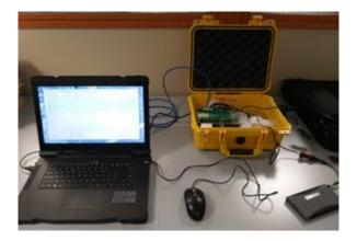
Figure 123 The present "portable" magnetic sensor prototype
