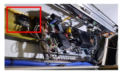
Figure 118 Preliminary implementation of the board deployed for video-anomaly detection
